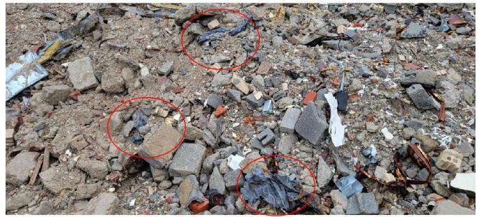
**Photo 6:** Lead sheeting near TP-12-2. Lead sample "VL-1" was collected of building debris surrounding sheeting for analysis of total lead and for toxicity characteristic leaching procedure (TCLP) analysis.
