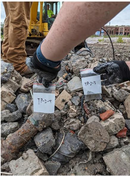
Samples TP-2-3 & 4, suspected Transite cement board and pipe joint insulation (Both samples found to contain asbestos)
