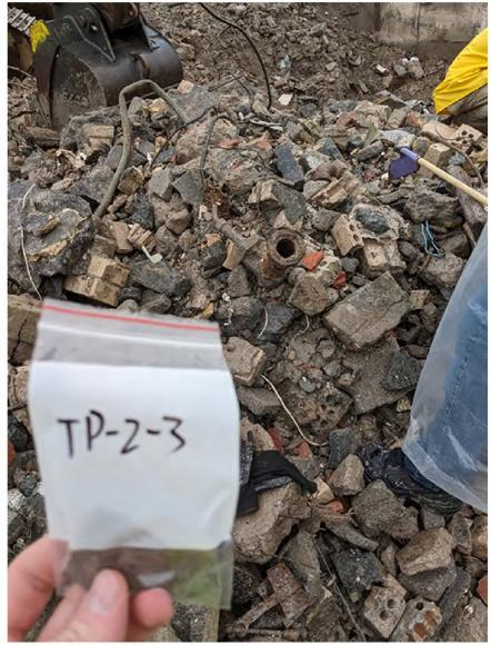
Samples TP-2-3, suspected Transite cement board (Sample found to contain Chrysotile asbestos)
