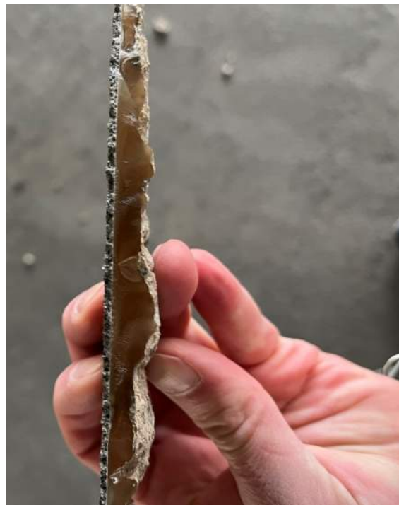
Photo 48: Epoxy overlay system cross section. Epoxy thickness is the result of going over highly scaled slab.
